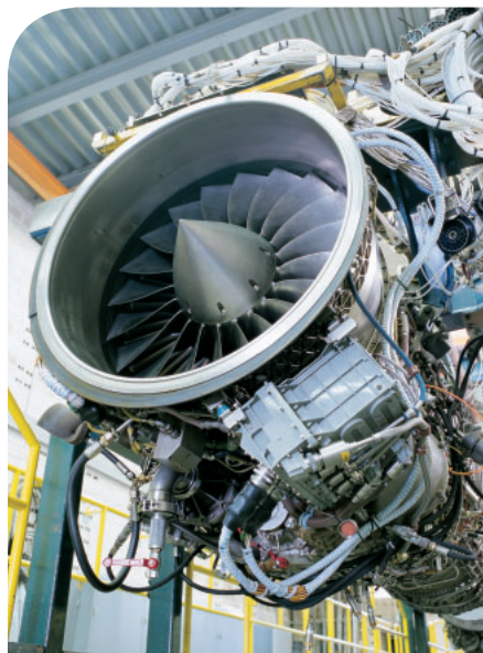
The EJ200, engine for the Eurofighter, is considered the most advanced engine in its class.
