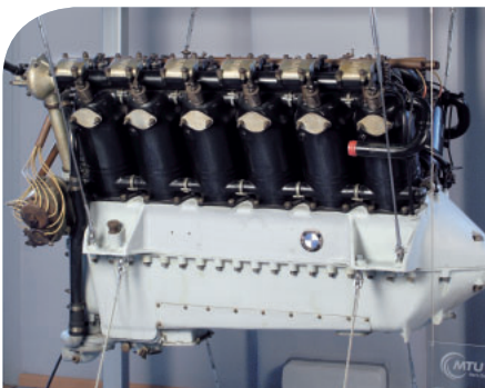
Standard engine of many historic German aircraft: the BMW VI.
