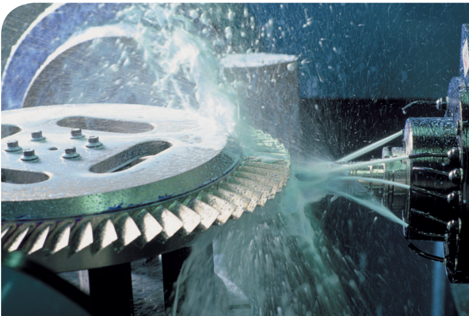
High-speed milling is one of the processes used in the production of blisks.
