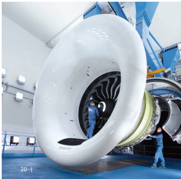
A GE90 on the test stand: MTU is known the world over for its testing and inspection expertise.
