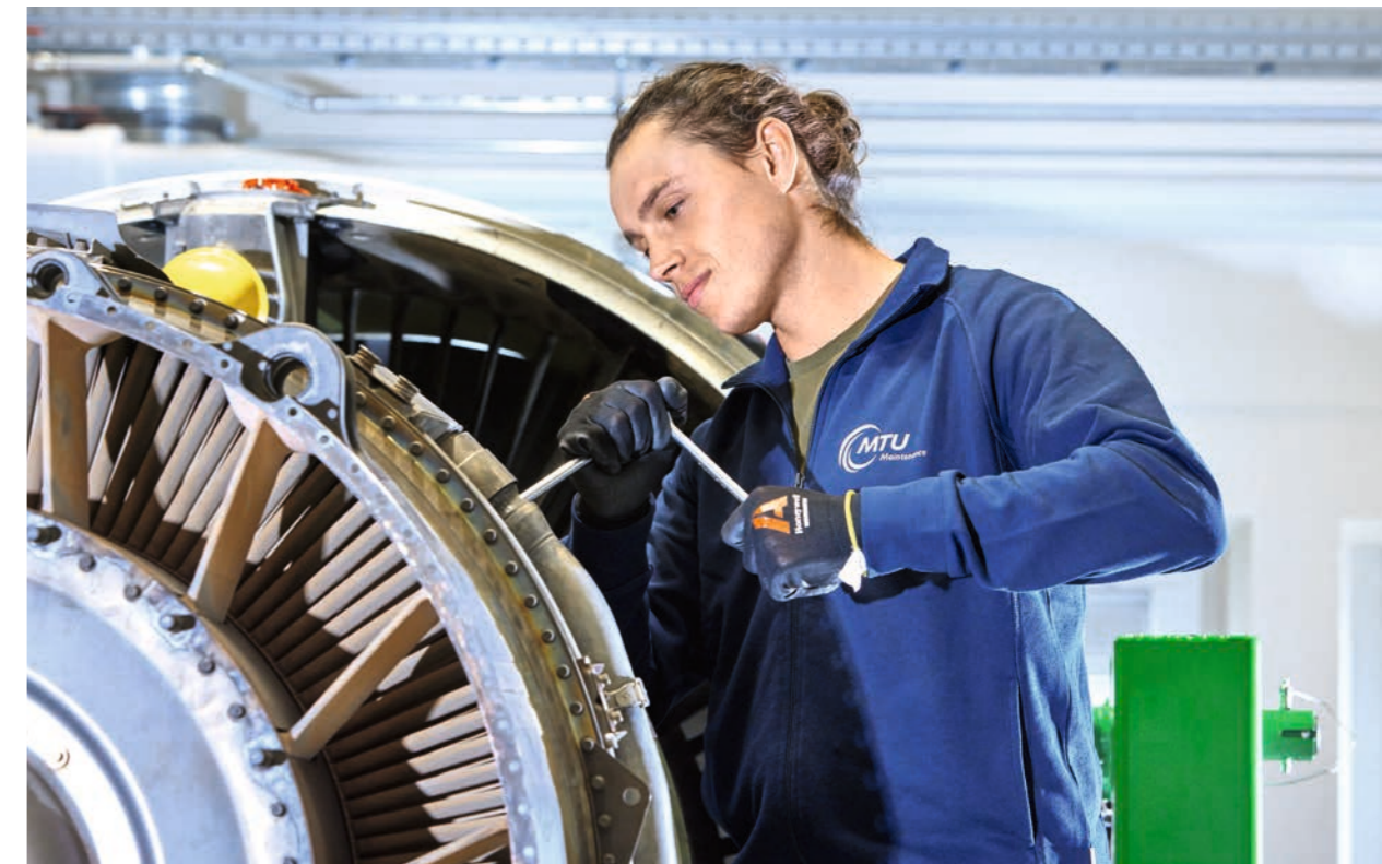
Assembly of a CFM56-7 engine: With its repair techniques, MTU Maintenance achieves globally unparalleled levels of restoration and long on-wing times.
