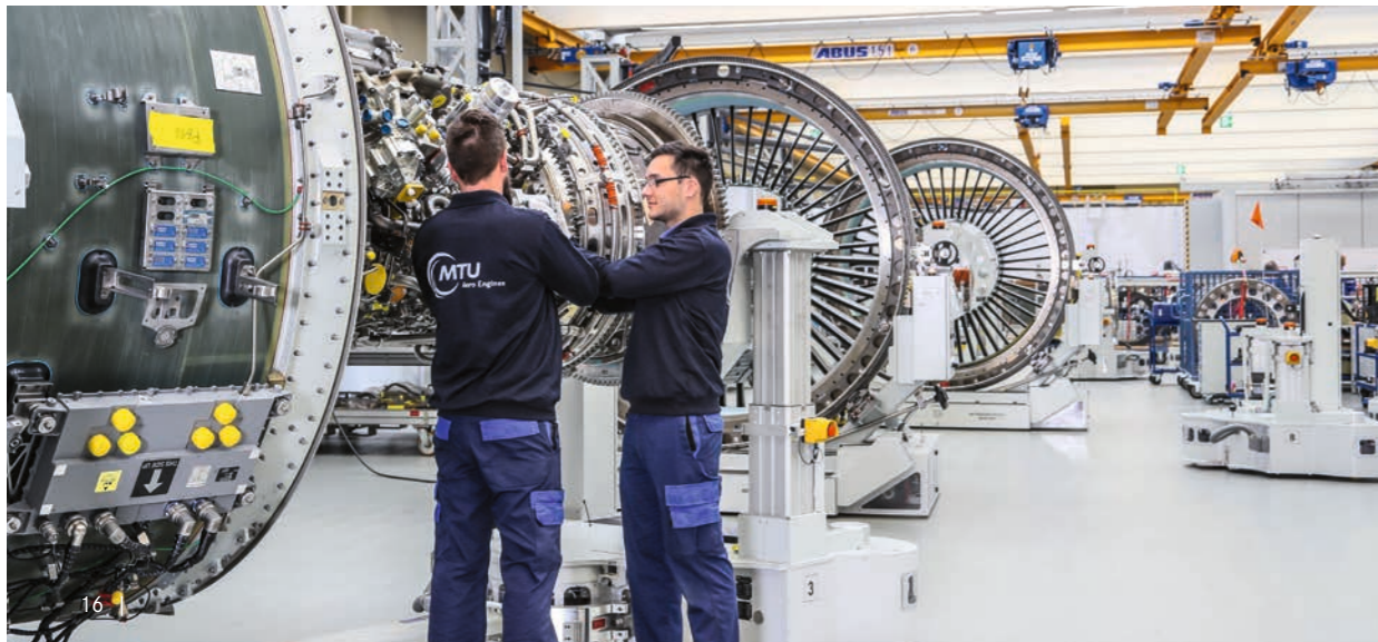
Geared for more power: MTU is responsible for the final assembly of one in three PW1 100G-JM engines for the A320neo.
