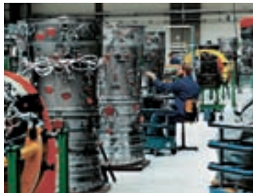
The RB199 Tornado engine is assembled by MTU in Munich for the German air force
