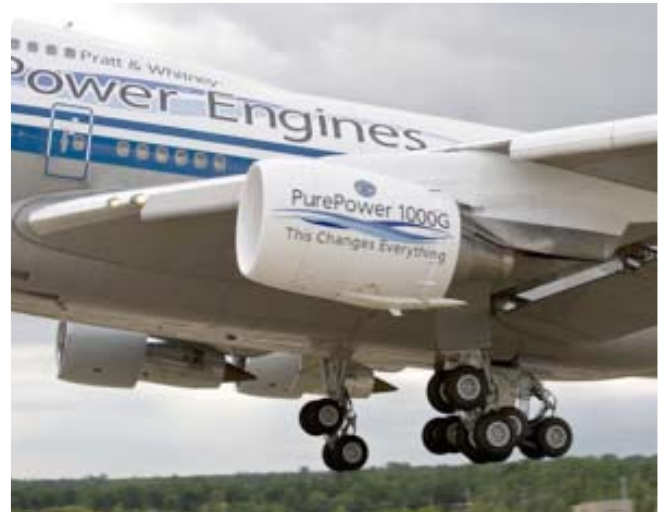
Picture: Geared turbofan demonstrator engine on the flying testbed of a Boeing 747
