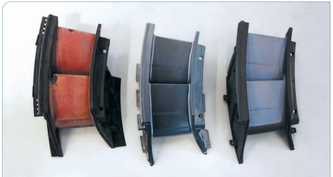
A high-pressure turbine vane getting a new lease on life: an engine-run vane (left), a vane after stripping (center) and a vane prepared for recoating (right).
