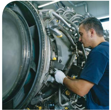
An LM2500 gas generator is assembled in MTU's shop.
