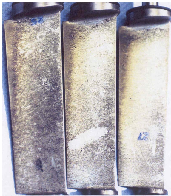
Vanes 25-27 without visible flow lines of contamination (concave sides)
