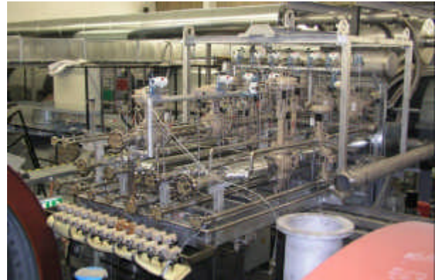
Fig. 5: Installation of the Secondary Air System (SAS) valve bay in front of the test cell
