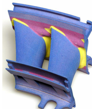
FIG. 4: First vane of cold flow rig with contoured endwalls
