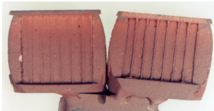
Fig. 7: Schematic of ceramic filled rails as advanced outer air seal concept.
