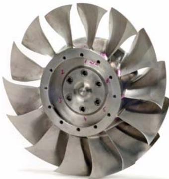
Figure 3 Rotor-3: Forward swept blisk
