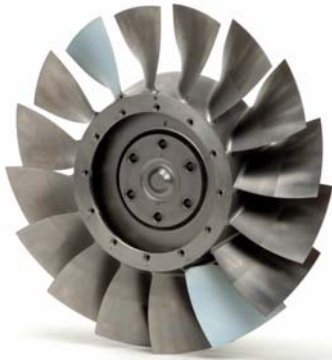
Figure 2 Rotor-1: Radially stacked blisk
