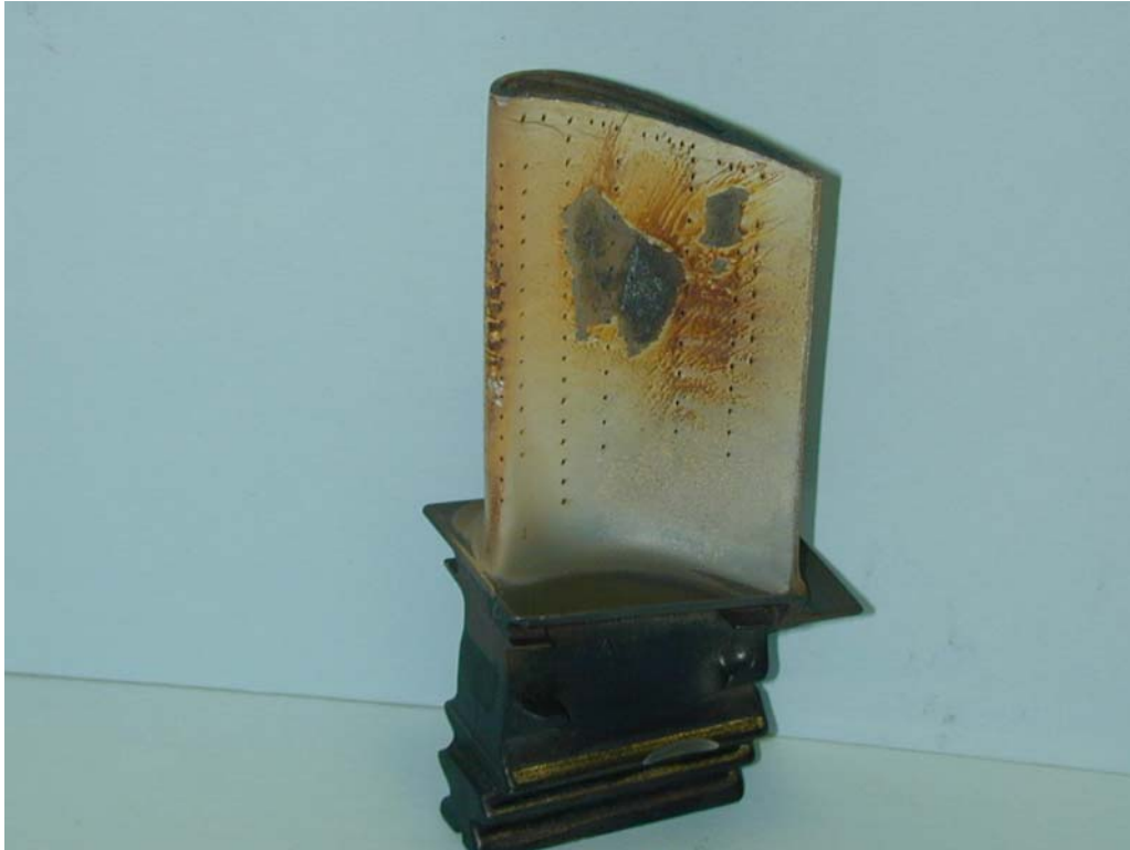
Figure7 : Incoming condition for repair of a stage 1 HPT blade
