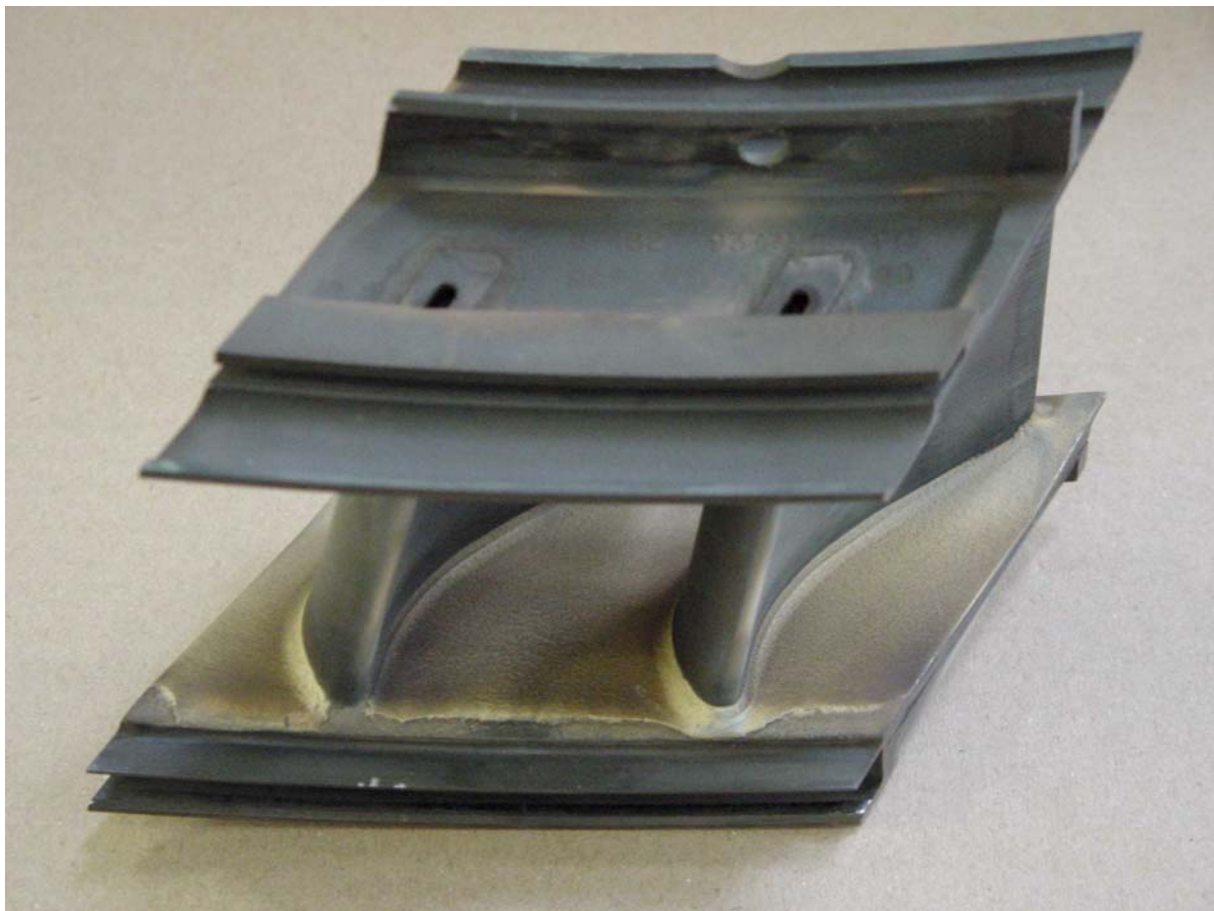
Figure4 : Incoming condition for repair of a stage 2 HPT Vane
