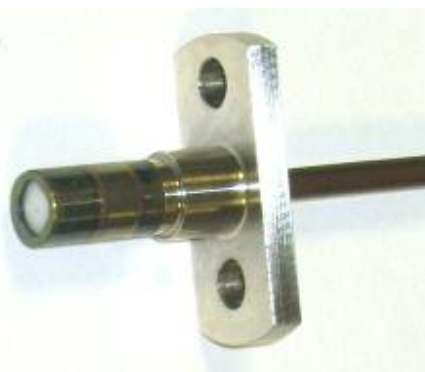
Fig. 14 Microwave tip clearance sensor and rig adapter
