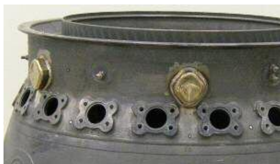
Fig. 5 Boss added by LMD to a used combustor case
