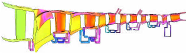
Fig. 6: Optimum Aerodynamic Stage Loading by Advanced CFD-Techniques
