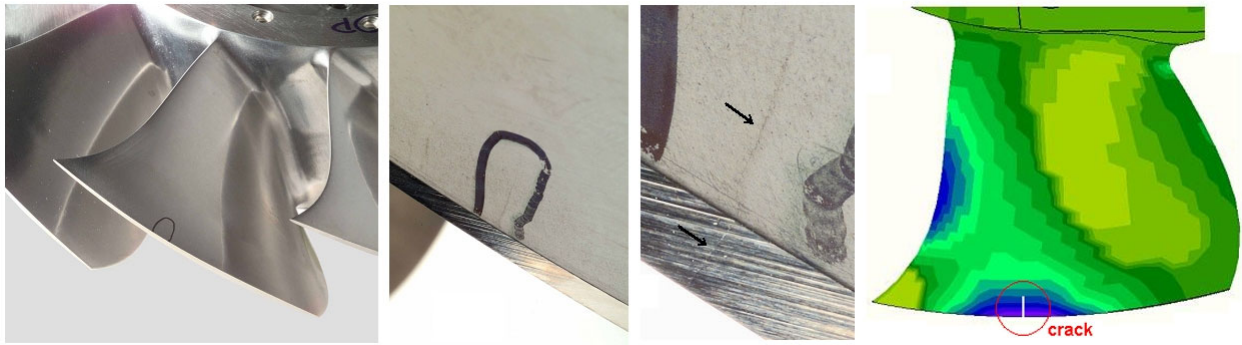
Figure 7: Cracked blade (left) and theoretical 1T stress distribution on the blade (right)
