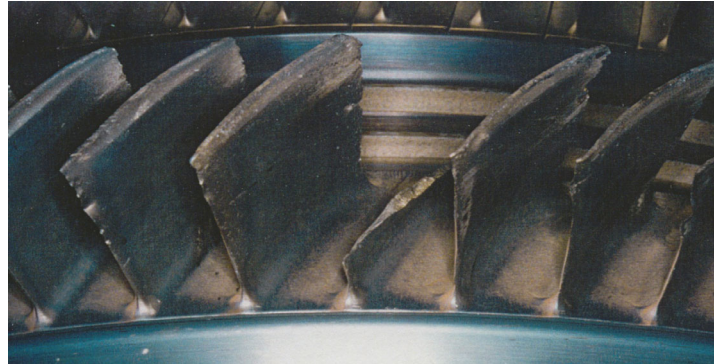
Figure 1: Severe damage to an axial-flow compressor following the loss of a blade
