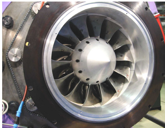
Figure 4: Single-stage compressor rig with blisk rotor
