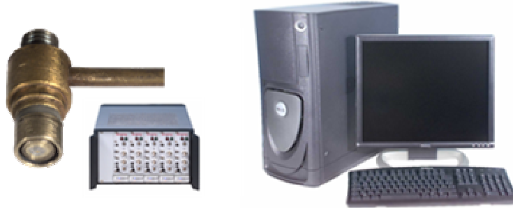
Figure 3: Latest BSSM system using capacitive probes and software triggering
