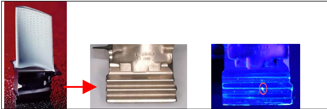
Fig. 7. CF6 turbine blade (specimen No. 2) with close-up view of blade root and FPI crack indication
