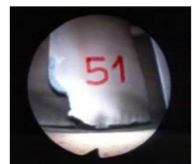
Figure 9 Vibration cause HPT blade deterioration
