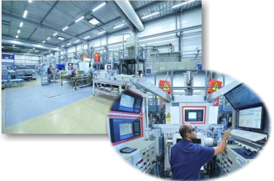
Fig. 2: EB-PVD coater at CCC in service
