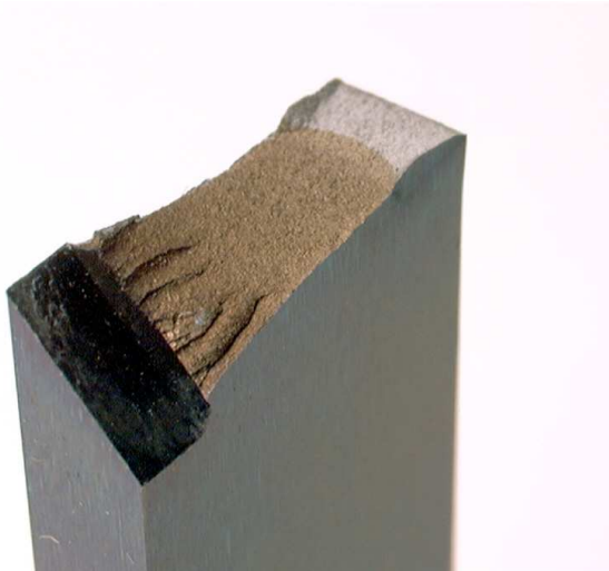
Figure 27 : Crack propagation in a titanium four-point bending specimen
