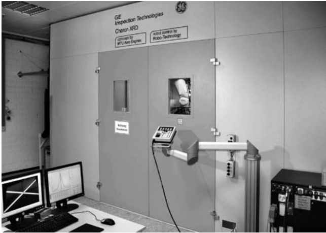
Fig. 1. Operator control stations in front of the closed Charon XRD X-ray protection and safety cabin.
