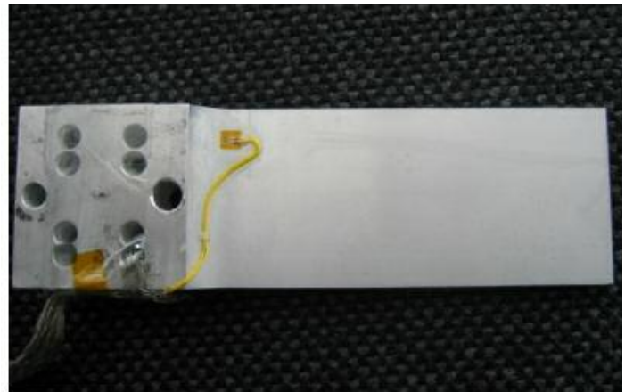
Fig. 4: Drawing and photograph of the test specimen, the applied strain gauge can be seen in the photograph
