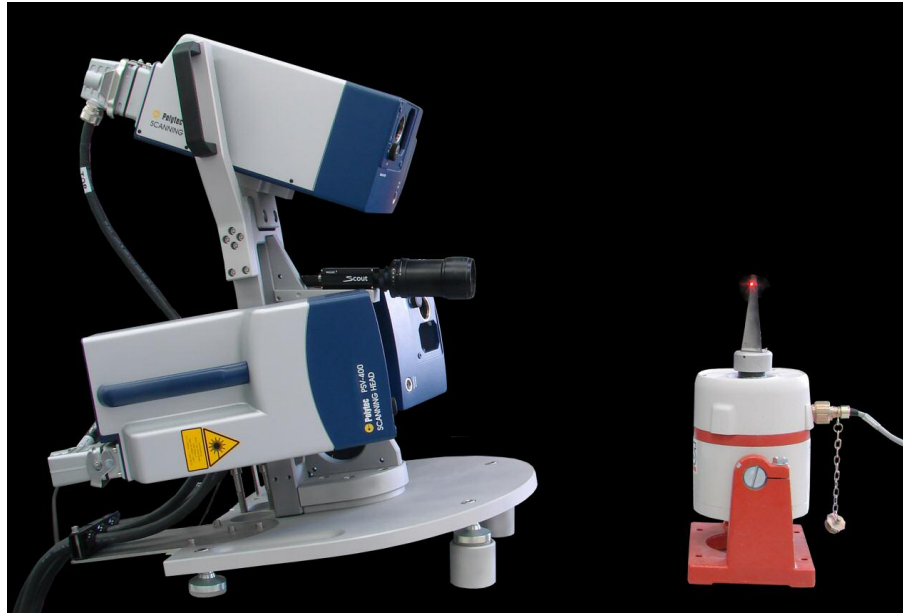
Fig. 1: Test setup comprising the three scanning heads and a digital camera (left) and a test specimen, mounted on an electromagnetic shaker (right)
