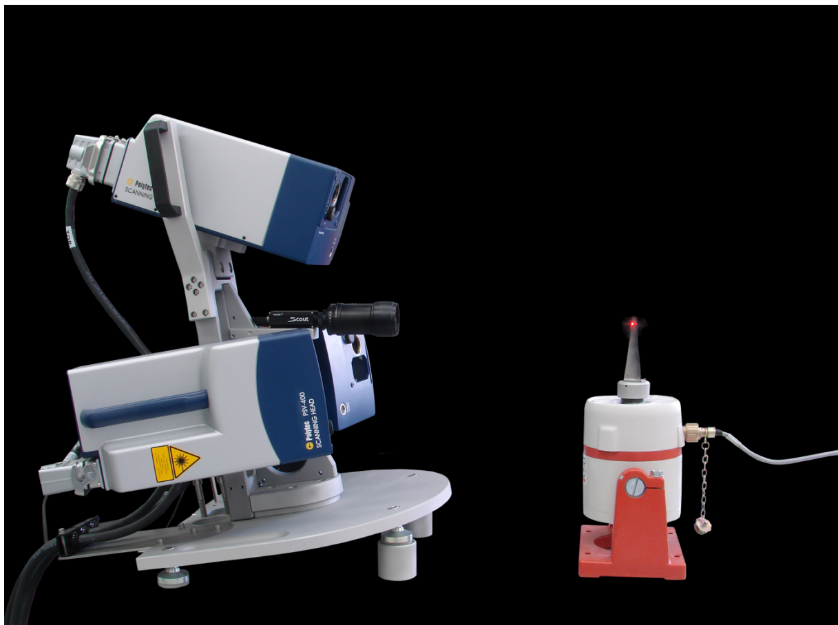
Fig. 2: 3-D Scanning Vibrometer testing a turbine blade.
