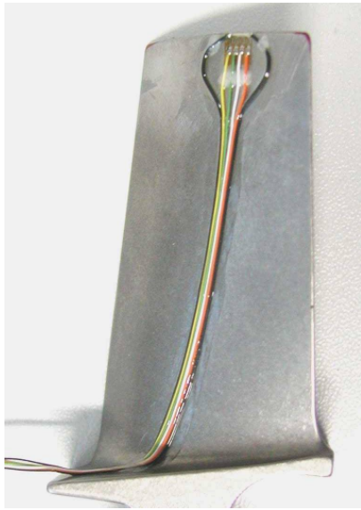
Fig. 1: Instrumented turbine blade with strain gauges.
