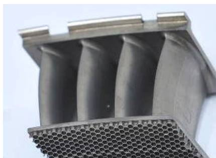
Figure 12: Compressor vane segments with integrated honeycombs (IN718)
