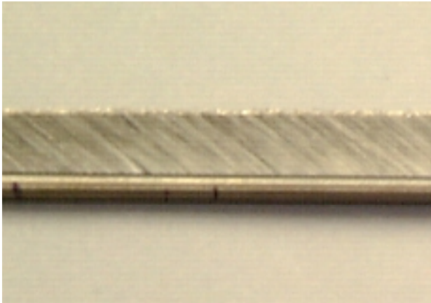
Fig. 3: Semi-finished Brush Seal strip
