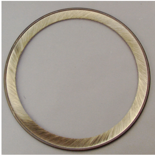
Fig. 4: Photograph of a Brush Seal core element
