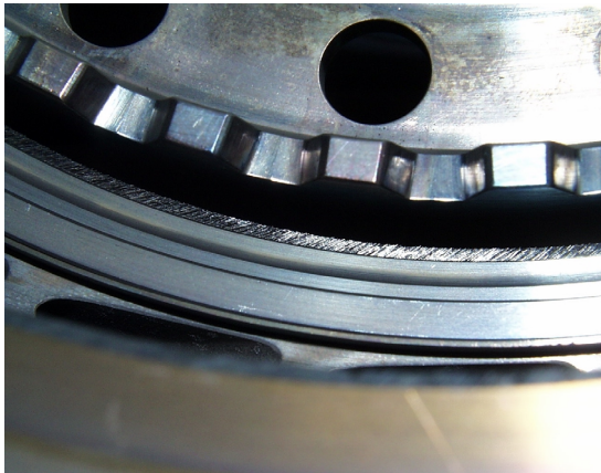
Fig. 7: MTU Brush Seal after 356 hrs. flight testing in a military project
