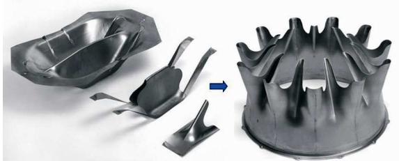
Figure 6 Manufacture of a mixer by laser cutting.
