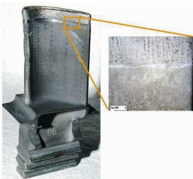
Figure 11 Single-crystal high-pressure turbine blade laser clad with a cobalt material with a transverse micro-section through the transition area.
