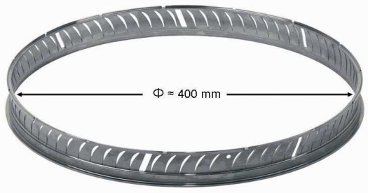
Figure 7 Laser cut shroud for the manufacture of compressor vane segments in IN718 material.
