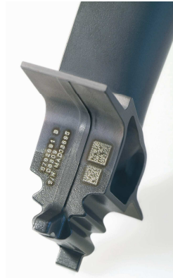
Figure 2 Laser marked low-pressure turbine blade.
