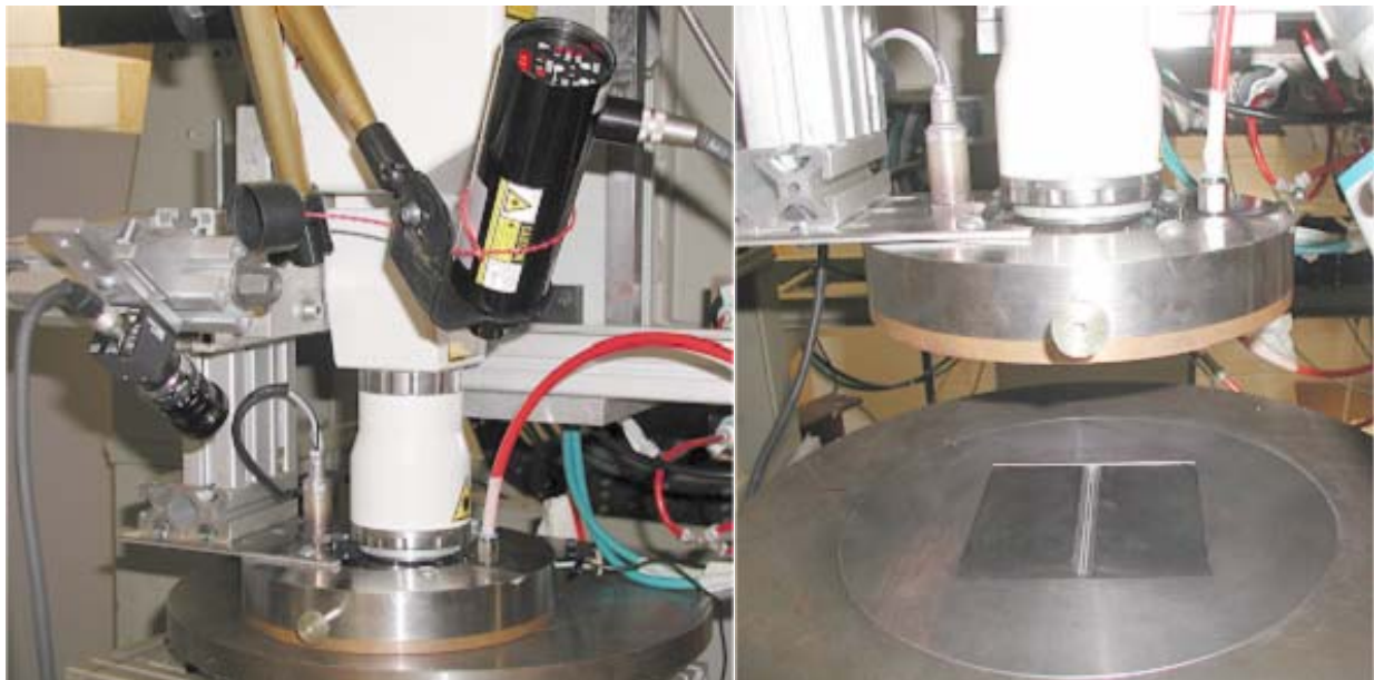
Figure 1 Experimental setup with Rofin DL025S high power diode laser, special gas chamber and different sensors
