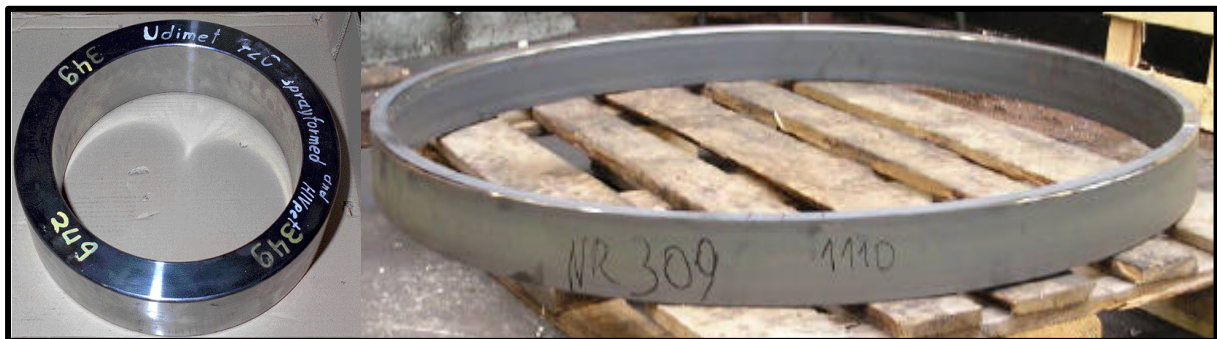
Figure 15. Component prototypes produced using the simplest (on Udimet 720) and most complex (on IN 718) post processing routes.
