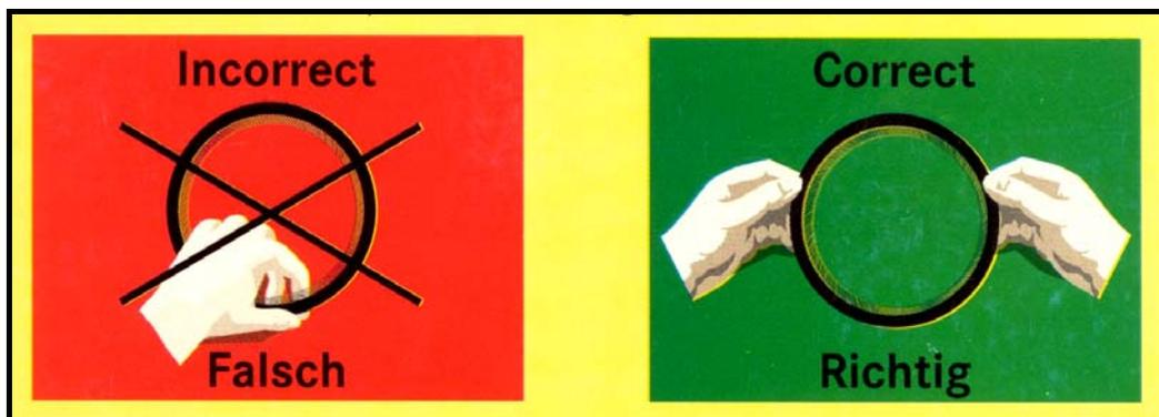
**Figure 1. Handling of the MTU brush seal**
