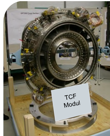
Assembly Turbine Center Frame
