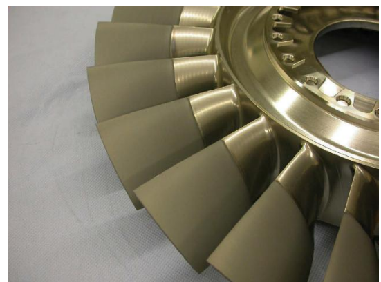
F9: Blisk treated with the ERCoat nt process (source: MTU Aero Engines)
