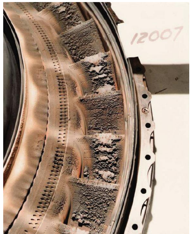
F5: Turbine blades with a crust left behind by molten volcanic ash (source: MTU Aero Engines)
