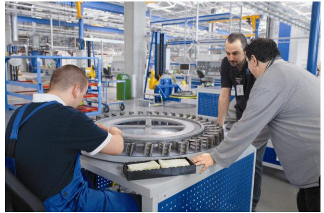
F4: Assembly of engine blades (source: MTU Aero Engines)
