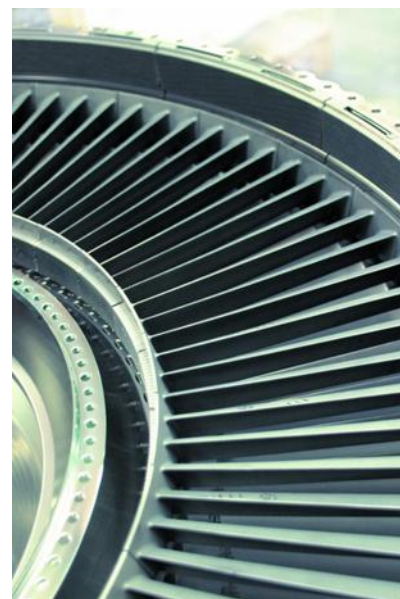
F2: Level-two components: vanes installed in the low-pressure turbine of a V2500 (source: MTU Aero Engines)
