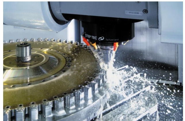
F2: Use of cooling lubricants during a deburring-milling process (source: MTU Aero Engines)
