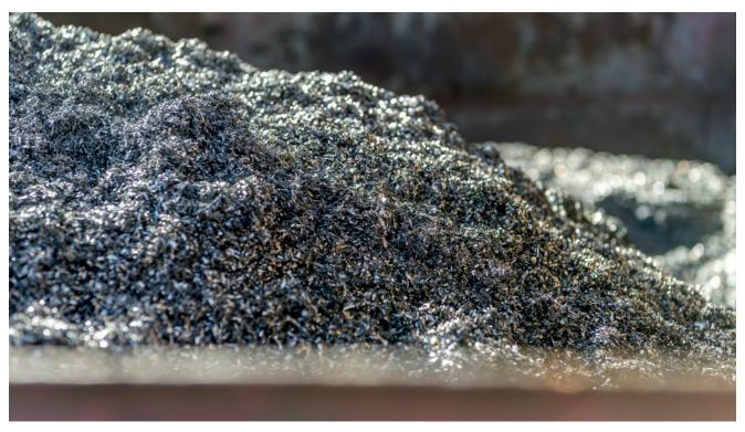
Valuable waste: MTU takes great care to separate metals by type. In this way, high-value chips can be returned to the cycle.
